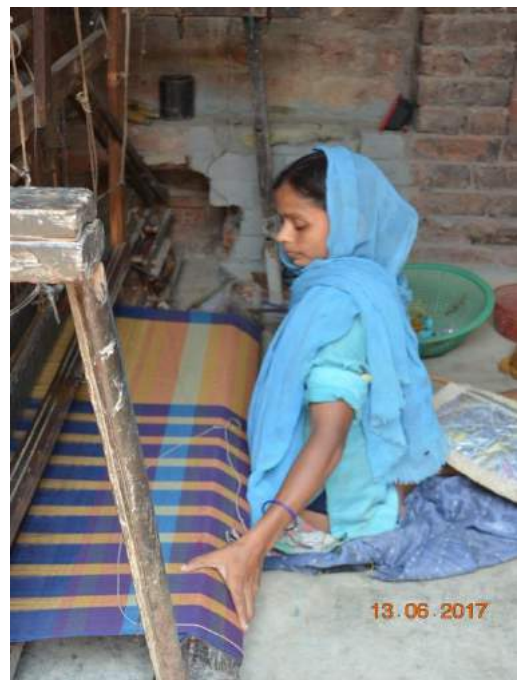
A woman weaver at the pit-loom weaving a cotton saree in Baragaon village, Barabanki district, Uttar Pradesh, India
